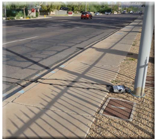
Automated bicycle counter installed on 44th Street, north of Thomas Road.
